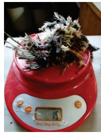
Fig. 7. Result of a 99 g feathered quail impact at 250 km/h on the combined barrier system: A – force-time graph; B – residue on the honeycomb fragment; C – mass of residue remaining on the honeycomb; D – small residue remaining on the Dyneema mesh.
