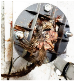
Fig. 7. Result of a 99 g feathered quail impact at 250 km/h on the combined barrier system: A – force-time graph; B – residue on the honeycomb fragment; C – mass of residue remaining on the honeycomb; D – small residue remaining on the Dyneema mesh.
